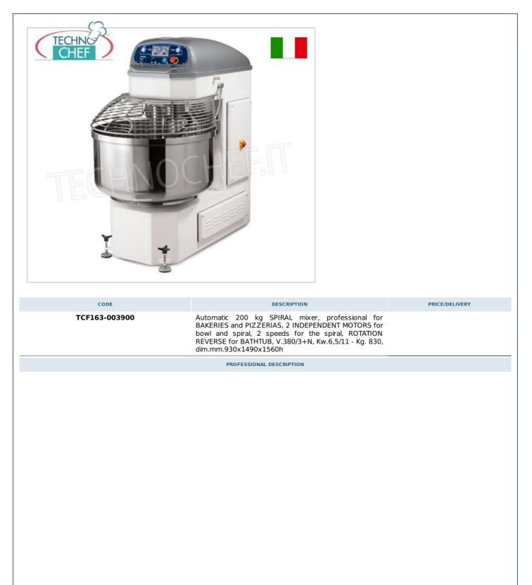
AUTOMATIC SPIRAL MIXER for 200 Kg of dough (290 liter bowl) , with FIXED HEAD and BOWL , 2 SPEED , 2 independent MOTORS for SPIRAL and BOWL :
